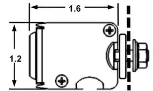
We also include two L-Brackets to facilitate mounting. These are optional and do not need to be used.
